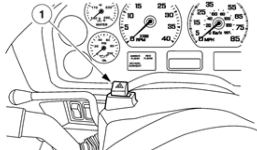
1. Hazard warning light switch
